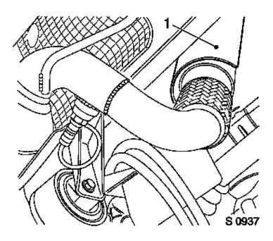
Catalytic converter from intermediate pipe -3 nuts (1).
