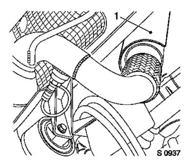
Wiring harness through wheelarch liner.
