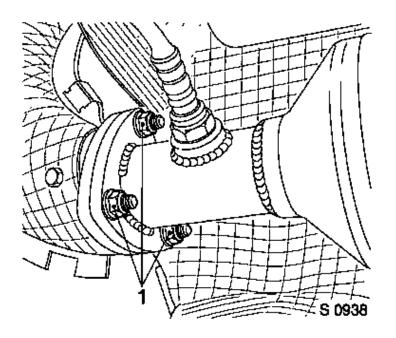
Lower heatshield (1) to exhaust manifold - 3 bolts, clip.
