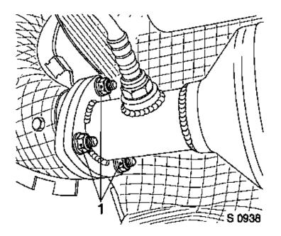
Catalytic converter from exhaust manifold – 3 nuts (1).
