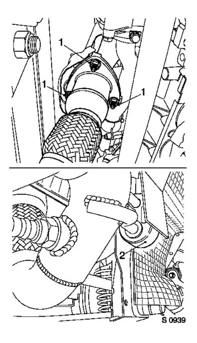
Catalytic converter to intermediate pipe -3 nuts (1).
